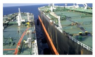
The overall safety for any STS operation depends on the use of correct size and number of fenders and certified tested hoses.
